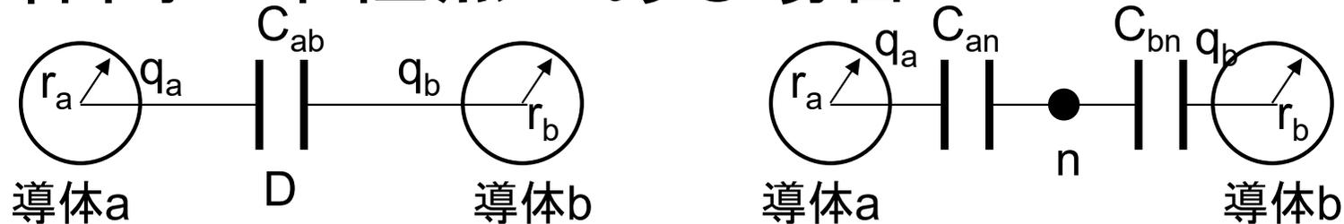
$$C_n = C_{an} + C_{bn} = 2C_{ab} = \frac{2\pi\epsilon}{\log_e \frac{D}{r}} \quad F/m$$
