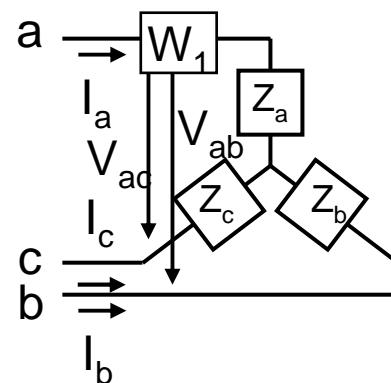
$$P_{ab} = V_{ab} I_a \cos(30^\circ + \phi)$$
