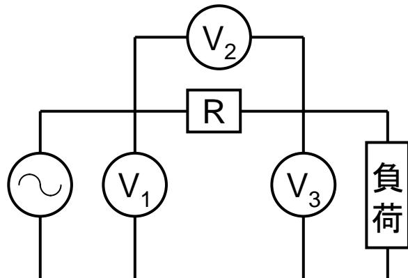
$$P_a = \frac{1}{2R} (V_1^2 - V_2^2 - V_3^2)$$
