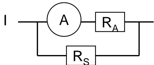
$$I = \frac{r_A + R_S}{R_S} I_A = m_A I_A$$
