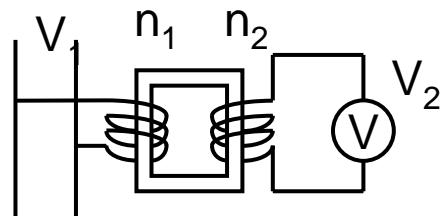
$$v_1 = \frac{n_1}{n_2} v_2 \quad \begin{array}{l} v_1: \text{測定電圧}, v_2: \text{指示電圧}, \\ n_1: \text{一次巻線数}, n_2: \text{二次巻線数} \end{array}$$
