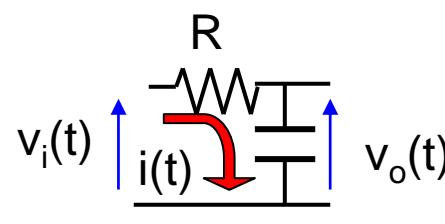
$$\begin{cases} v_i(t) = Ri + \frac{1}{C} \int i dt \\ v_o(t) = \frac{1}{C} \int i dt \end{cases} \quad \Rightarrow \quad \begin{cases} V_i(s) = RI(s) + \frac{I(s)}{sC} \\ V_o(s) = \frac{I(s)}{sC} \end{cases} \quad G(s) = \frac{V_o(s)}{V_i(s)} = \frac{1}{sCR + 1}$$
