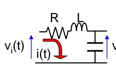
$$\left\{ \begin{array}{l} v_i(t) = Ri + L \frac{di}{dt} + \frac{1}{C} \int i dt \\ v_o(t) = \frac{1}{C} \int i dt \end{array} \right. \quad \rightarrow \quad \left\{ \begin{array}{l} V_i(s) = RI(s) + sLI(s) + \frac{I(s)}{sC} \\ V_o(s) = \frac{I(s)}{sC} \end{array} \right.$$
