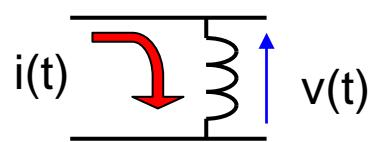
$$v(t) = L \frac{d}{dt} i(t) \quad \Rightarrow \quad V(s) = s L I(s)$$
