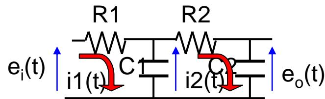
$$\begin{cases} e_i(t) = R_1 i_1 + \frac{1}{C_1} \int (i_1 - i_2) dt \\ \frac{1}{C_1} \int (i_1 - i_2) dt = R_2 i_2 + \frac{1}{C_2} \int i_2 dt \\ e_o(t) = \frac{1}{C_2} \int i_2 \end{cases}$$
