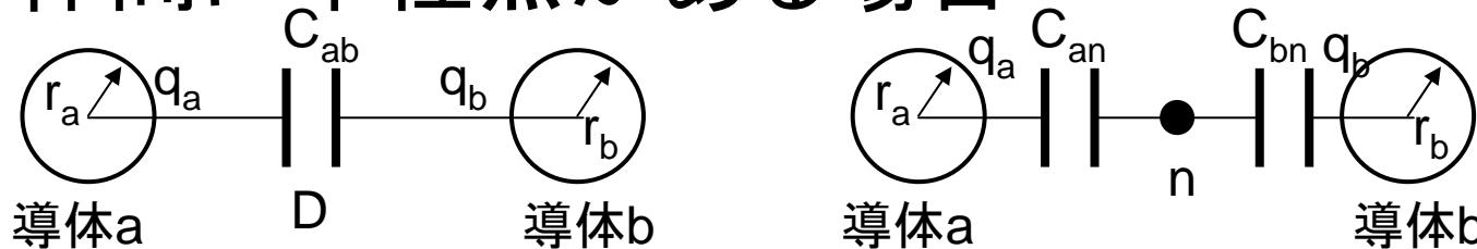
$$C_n = C_{an} = C_{bn} = 2C_{ab} = \frac{2\pi\epsilon}{\log_e \frac{D}{r}} F/m$$
