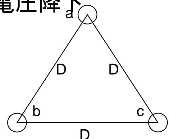
$$V_{ab} = \frac{1}{2\pi\epsilon_0} \left( q_a \log_e \frac{D}{r} + q_b \log_e \frac{r}{D} \right) V$$
