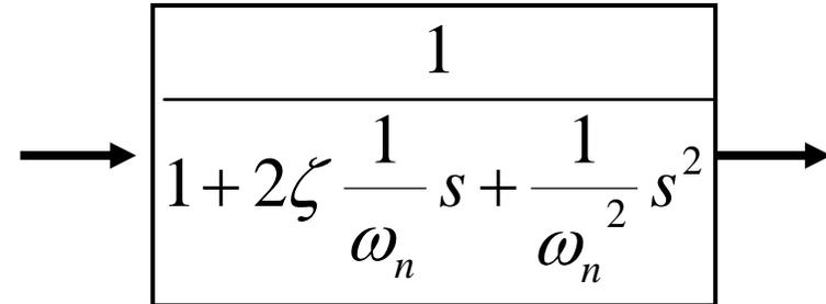
$$G(j\omega) = \frac{1}{1 + 2\zeta \left( j \frac{\omega}{\omega_n} \right) + \left( j \frac{\omega}{\omega_n} \right)^2}$$
