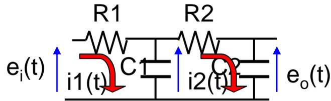
$$\begin{cases} e_i(t) = R_1 i_1 + \frac{1}{C_1} \int (i_1 - i_2) dt \\ \frac{1}{C_1} \int (i_1 - i_2) dt = R_2 i_2 + \frac{1}{C_2} \int i_2 dt \\ e_o(t) = \frac{1}{C_2} \int i_2 dt \end{cases}$$
