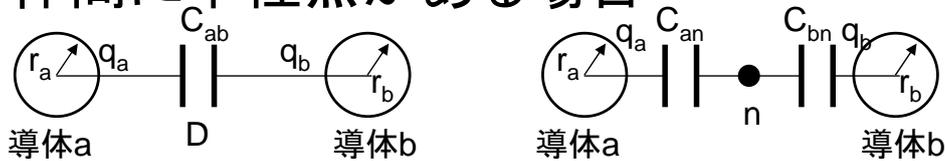
$$C_n = C_{an} = C_{bn} = 2C_{ab} = \frac{2\pi\epsilon}{\log_e \frac{D}{r}} \quad F/m$$
